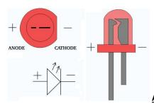
ALWAYS put a 220R, 470R or up to a 1K resistor in series with an LED to help
