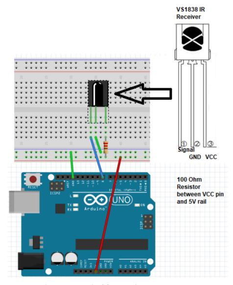
Connect Arduino pin 8 to the 'S' pin on the VS1838 receiver.
