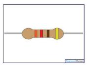
Resistors are NOT directional. Current can flow in both directions.
